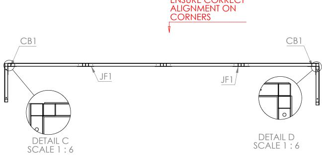
**Step 2** Attach **ST15** Tie bars to **SC** frames using **CB1** Brackets. Fix the **ST3** Tie bars to the **ST15** bars using **CB1** Brackets and attach to the **P5** Post using the **JFT** bracket.
