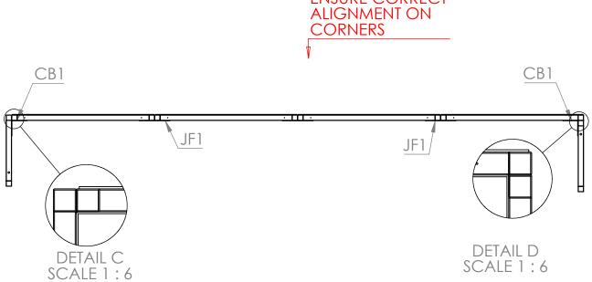
**Step 2** Attach **ST15** Tie bars to **SC3** frames using **CB1** Brackets. Fix the **ST3** Tie bars to the **ST15** bars using **CB1** Brackets and attach to the **P5** Post using the **JFT** bracket.
