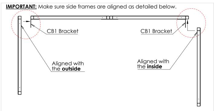
**Step 2** Attach front **S1** frame and **ST1** tie bar using **CB1** brackets in the corners and **JF1** brackets on the straight joints.
