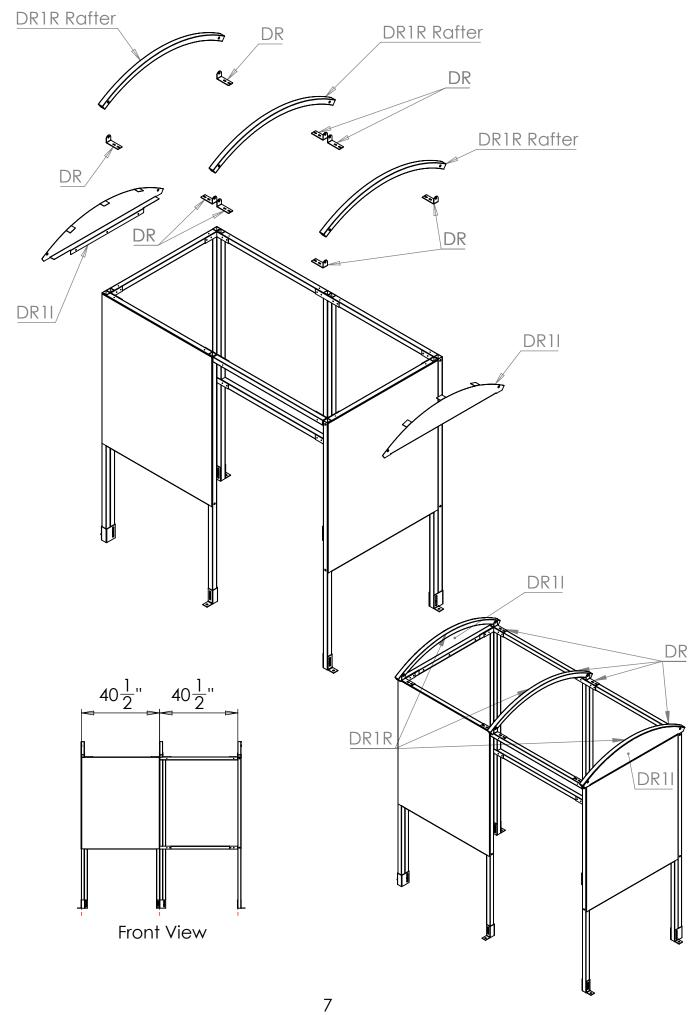
Step 4 Stick sealing strips on top of rafters and install roof sheets. Seal the central gap and edges with a **DR1T** strip. Install the **DRAT2** Angle trim to the bottom of the roof panels. Then fit the black plastic caps on exposed nuts and bolts.
