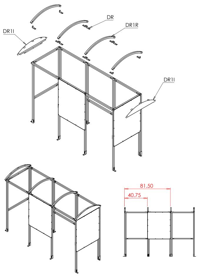
**Step 4** Place **DR1PO** and the **DR1PI Panels** on top of the rafters. Follow the order shown below. Secure the panels using the **DRATO** and **DRATI** angles. These are secured with the 1.5" Tech screws.
