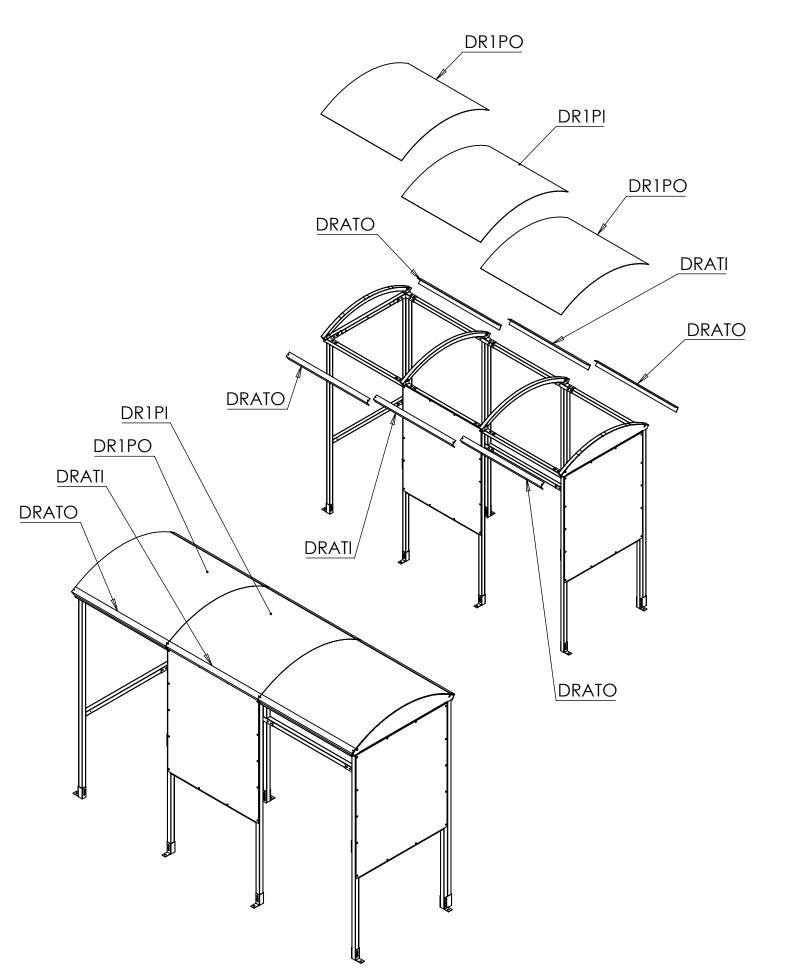
**Step 5** Attach the **DR1T** Strips by screwing throught the panels and into the rafters using 1.5" Tech screws, then attach the **DR1PO** and **DR1PI** Trims to the outer/lower edges of the panels.
