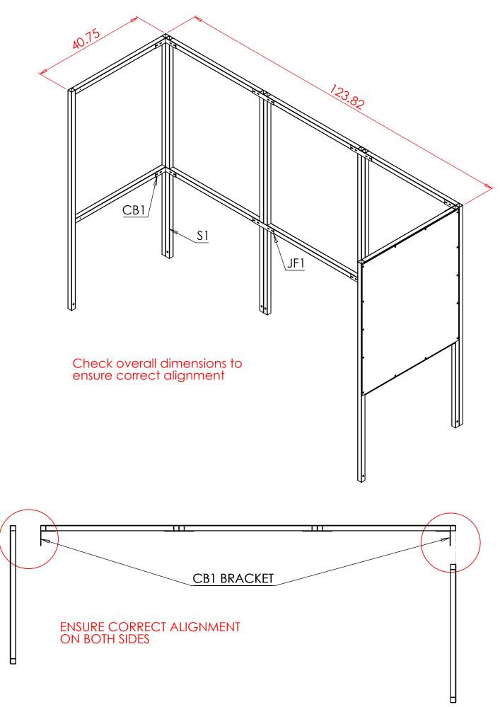
**Step 2** Attach **ST1** Roof Ties and final **S1** to the structure using **CB1** and **JF1** Brackets.
