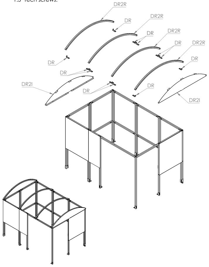
**Step 3** Align the **DR2PO** roof panels with the outer roof rafters and equaly space the **DR2PI** panel in the middle. Then use the DRATO and DRATI angles to attach the bottom of the panels with 1.5" Tech screws.
