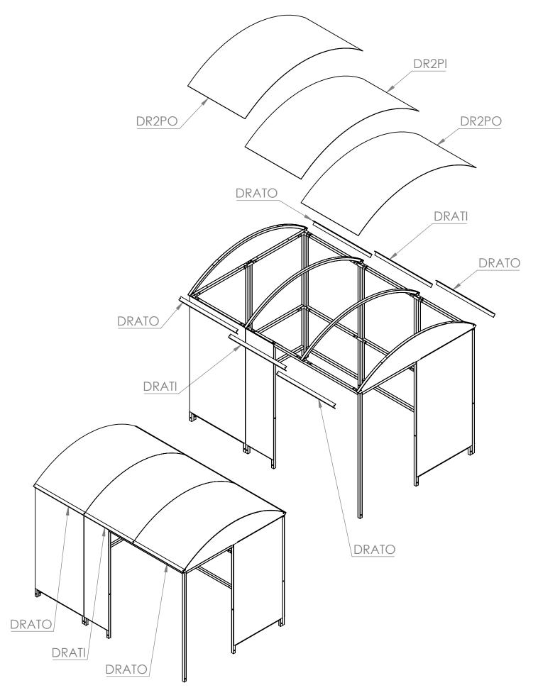
**Step 4** Attach the **FT1** and **FT3** foot brackets to the frames. Make sure the shelter is square and in its desired position before using the anchor bolts to fix it to the the ground. Screw down the **DR2T** directly into the rafters as shown below, using 1.5" Tech screws.
