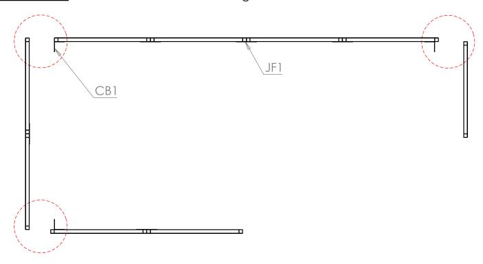
**Step 2** Attach front **S1** frame and **ST3** tie bar using **CB1** and **JF1** brackets.
