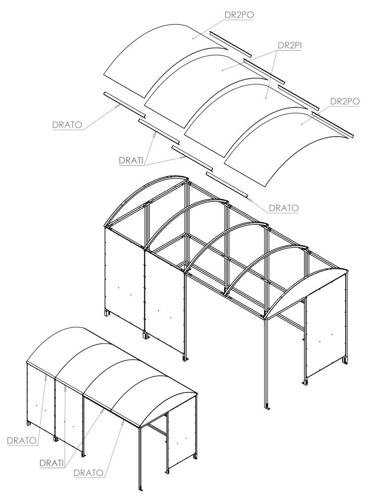
Step 5 Seal the central gaps and edges with the DR1T strips. Once the shelter is in its final position and squared up, attach the FT1 and FT3 foot brackets and use anchor bolts to secure everything to the ground. Finally fit the black plastic caps on exposed nuts and bolts.
