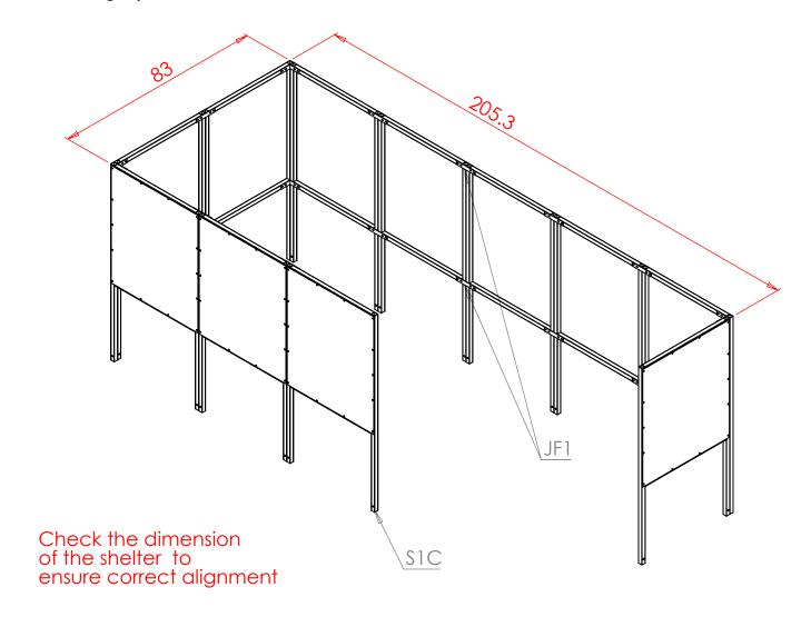
**IMPORTANT:** Make sure side frames are aligned as detailed below.
