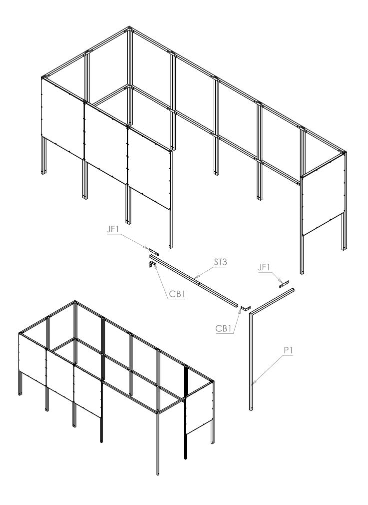
**Step 3** Secure the **DR1R** roof rafters into place using the **DR** Brackets. The **DR1I** infill panels are screwed into place using 1" tech screws but must be placed into position at the same time as the end rafter.
