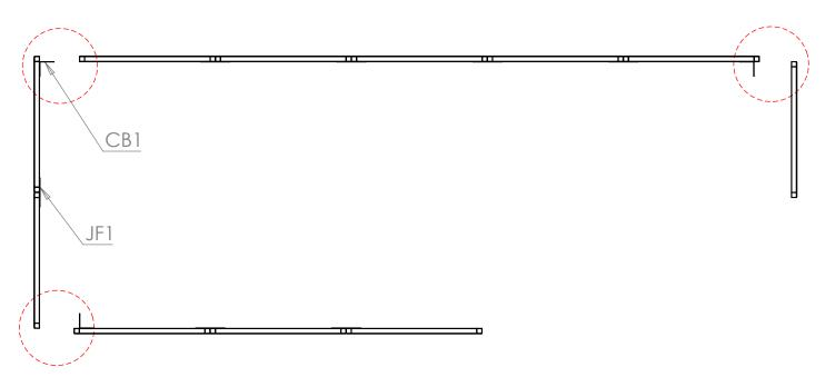
**Step 2** Attach the **ST3** tie bar ans **P1** post using **CB1** and **JF1** brackets.
