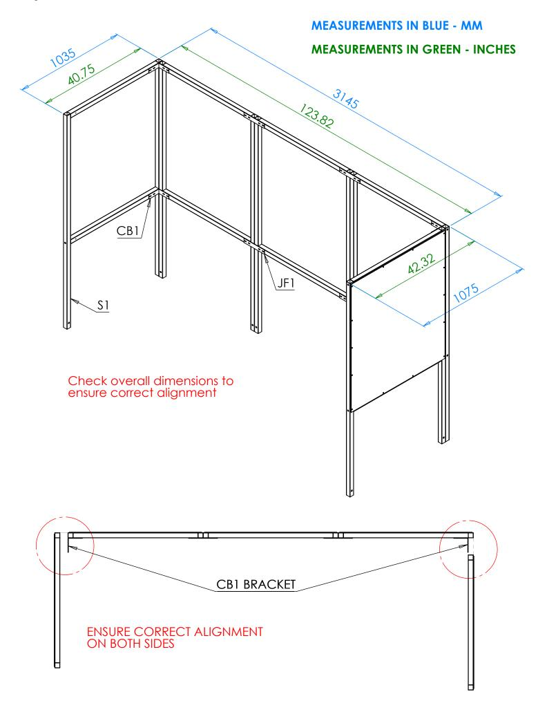
Step 2 Attach ST1 Roof Tie and final S1 to the structure using CB1 and JF1 Brackets.
