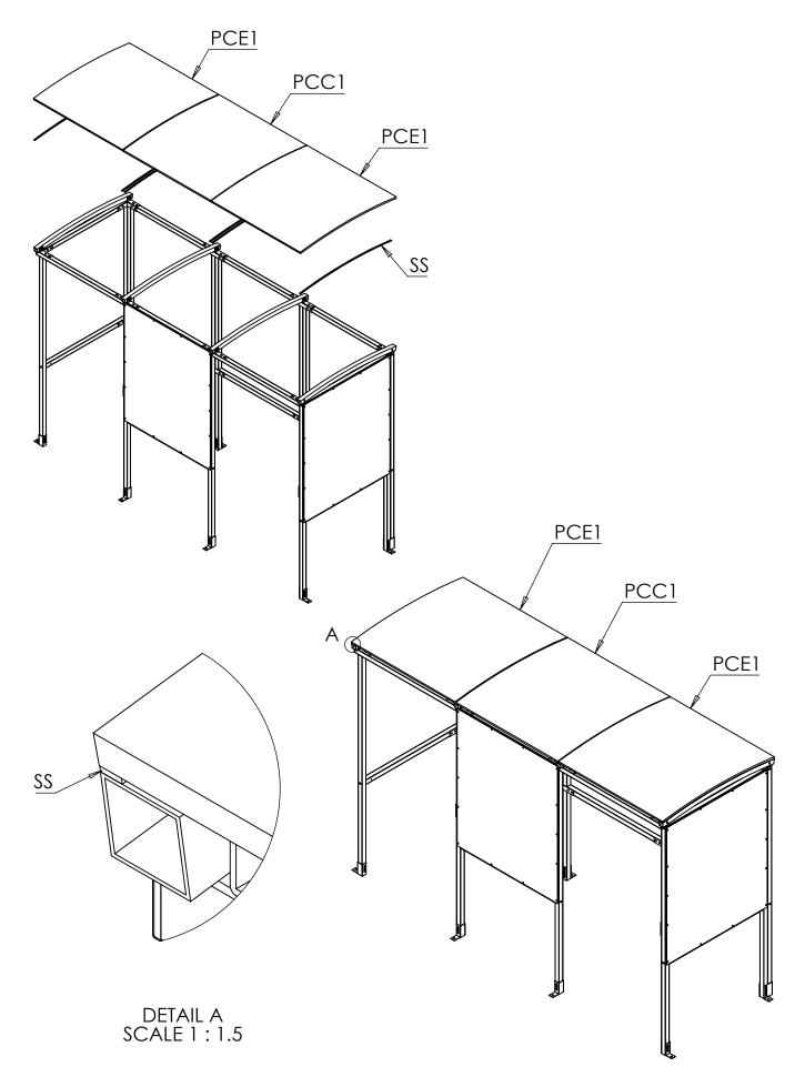
**Step 6** Secure panels in place using an **RC1 Strip** screwing through the panels and into the rafters using **38mm Tech screws**, then attach the **2MD Edge Trim** to the outer edges of the panels, tapping them on with a mallet. Then fit the black plastic caps on exposed nuts and bolts. Fit the square plastic end caps (**EC40**) to any open ends of box sections.
