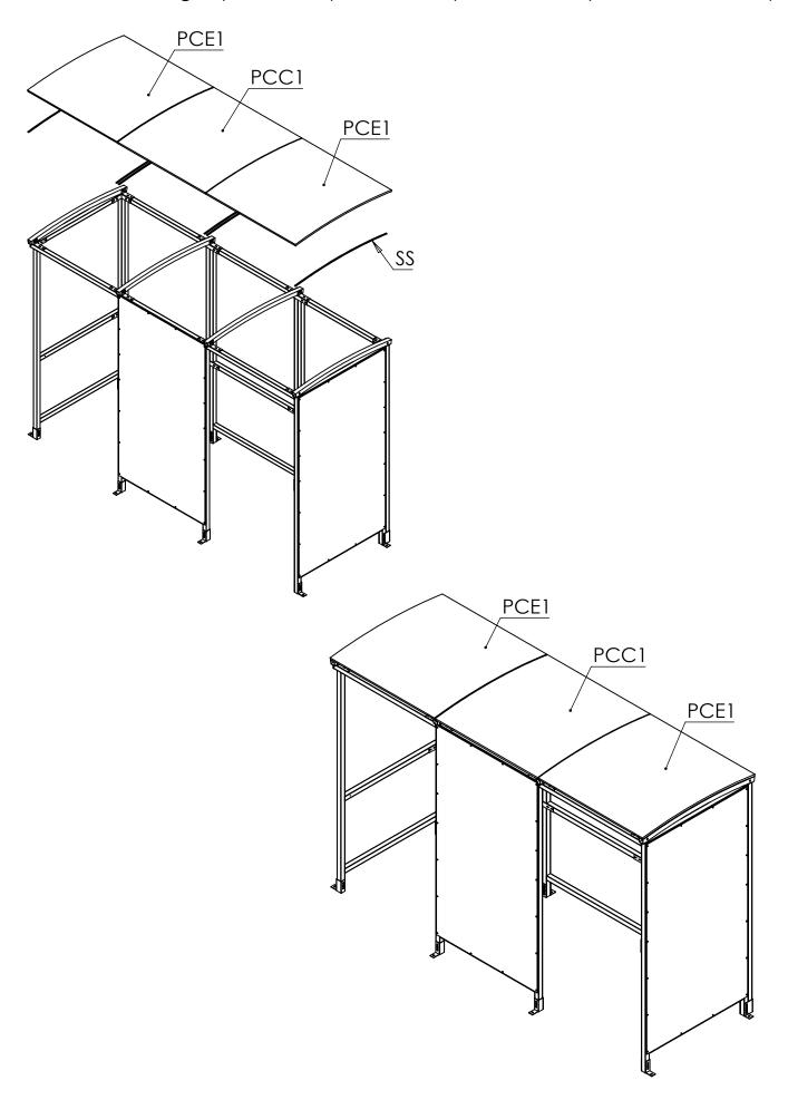
**Step 6** Secure panels in place using an **RC1 Strips**, screwing through thepanel and into the rafter **38mm Tech screws**, then attach the **2MD** Edge Trim to the outer edges of the panels, tapping them on with a mallet. Then fit the black plastic caps on exposed nuts and bolts. Fit the square plastic end caps to any open ends of box sections.
