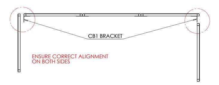
**Step 2** Attach **ST1** Roof Tie and final **S1C** to the structure using **CB1** and **JF1** Brackets.
