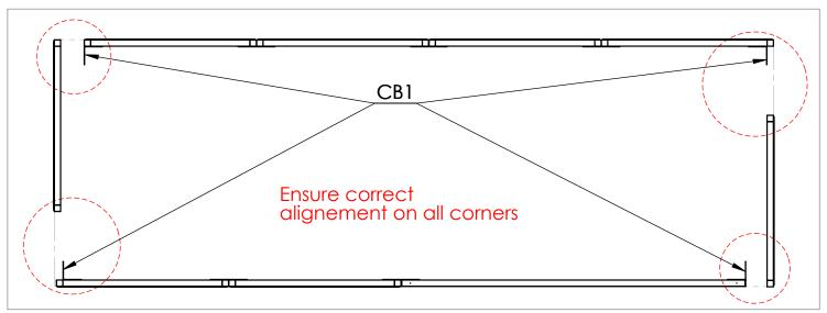
Step 2 Move the Shelter to its final position and attach all FT1 and FT3 foot brackets. Attach RB1 Brackets to the top of the frames and then bolt the R1 Rafters in place through them.
