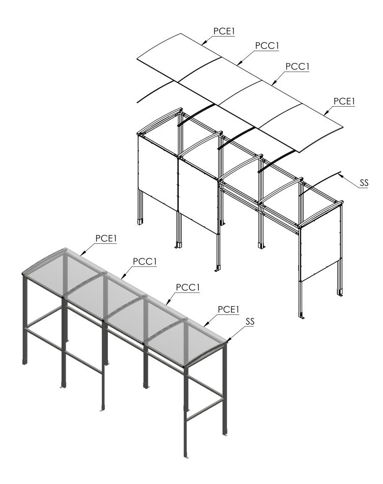
**Step 4** Secure the roof panels in place by drilling the **RC1** strips directly into the frame of the shelter using the **38mm screws.** Then apply the **2MD** edge trim along the bottom edges of the roof, tapping it in place using a mallet. Push fit the palstic end caps (**EC40**) into any open end of box section. Use the black plastic caps to fit over exposed nuts and bolts.
