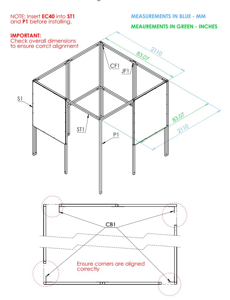
**Step 2** Move shelter in to its final position, make sure everything is square and secure to the floor using **FT1** and **FT3** foot brackets.
