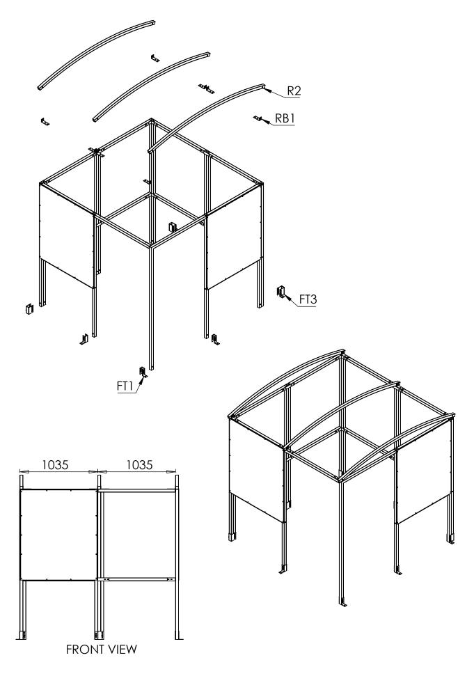
**Step 3** Apply **SS** sealing strips to the rafters (two for cental rafter) and line up the **PCE2** roof panels to the outside of the shelter, leaving a gap between them.
