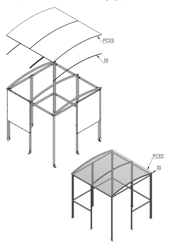
**Step 4** Apply **RC2** strips on top of the panels and use **38mm Tech screws** to secure them in place, drilling through the panels and into the rafters. Then clip on the **2MD** edge trim to the edges of the roof panels, tapping it on with a mallet. Then fit the Black plastic caps on exposed nuts and bolts. Fit the square plastic end caps (**EC40**) to any open ends of box sections.
