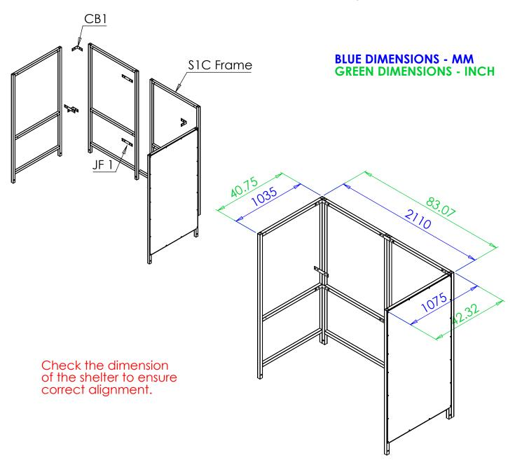
**IMPORTANT:** Make sure side frames are aligned as detailed below.
