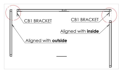
**Step 2** Insert **EC40** end caps into both ends of the **ST1** tie bar. Attach front **S1C** frame and **ST1** tie bar using **CB1** brackets in the corners and **JF1** brackets on the straight joint. Once the main structure is secured, move the shelter into its final position and install foot brackets **FT1** and **FT3** to fix shelter to the ground.
