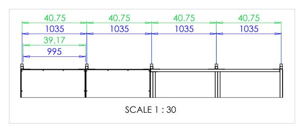
**Step 3** Apply **sealing strips (SS)** to the top of the rafters then arange the roof panels by lining up the end panels(**ACE1**) flush with the rafters and leaving a gap between the middle pieces(**ACC1**).
