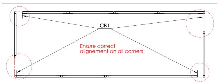
**Step 2** Move the Shelter to its final position and attach all **FT1** and **FT3** foot brackets. Then attach **R1** roof rafters using **RB1** brackets.
