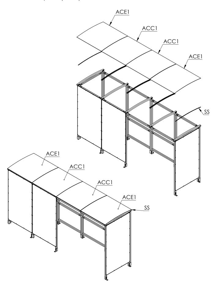
**Step 4** Secure the roof panels in place by drilling the **RC1** strips directly into the frame of the shelter using the **25mm Tech screws**.
