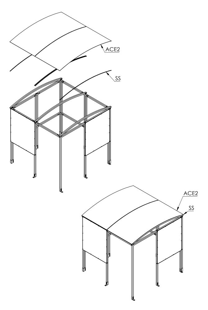
**Step 4** Apply **RC2** strips on top of the panels and use **25mm Tech screws** to secure them in place. Fit the Black plastic caps on exposed nuts and bolts. Fit the square plastic end caps to any open ends of box sections. Screw the **A1** Angles in place along the edges of the shelter as shown below.
