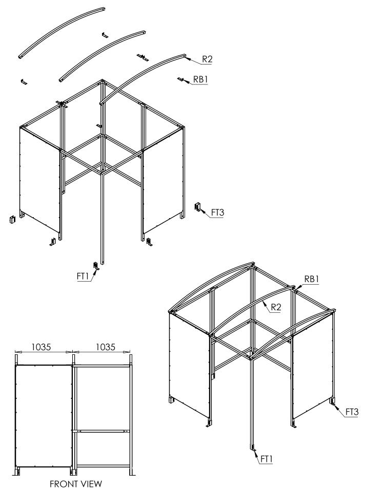
**Step 3** Apply **ss** sealing strips to the rafters (two for cental rafter) and line up the **ACE2** roof panels to the outside of the shelter, leaving a gap between them.
