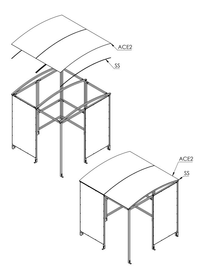
Step 4 Apply RC2 strips on top of the panels and use 25mm Tech screws to secure them in place. Fit the Black plastic caps on exposed nuts and bolts. Fit the square plastic end caps to any open ends of box sections. Screw the A1 Angles in place along the edges of the shelter as shown below.
