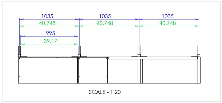
**Step 4** Stick sealing strips (**SS**) to the rafters. Align the **ACE2** roof panels with the outer roof rafters and equaly space the **ACC2** panel in the middle.
