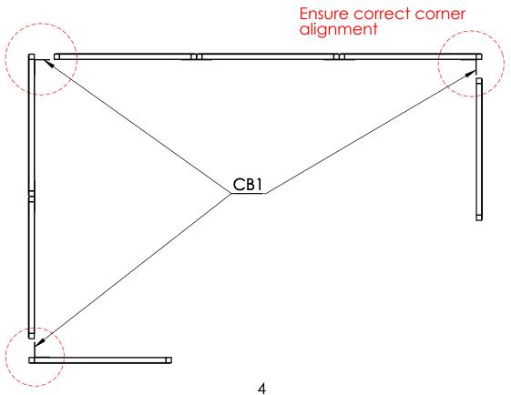
**Step 2** Attach **P1** post using a **JF1** bracket then use two **JF1** brackets to attach **S3C** frame. The **ST5** tie bar is mounted using a **CB1** and a **JF1** bracket. Make sure the structure is square then move the shelter to its final location before using the **FT1** foot brackets to secure it to the ground.
