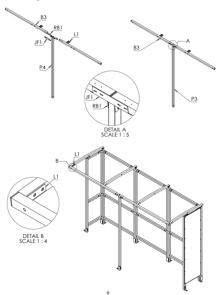
**Step 4** Attach the **FT1** and **FT3** foot brackets, Move the Shelter into its final position and make sure its square. Then use concrete anchor bolts to secure it to the the ground.
