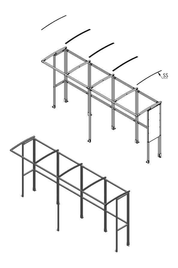
**Step 7** Place **ACE3** and **ACC3** with small gaps between each, Use **RC3** strips and screws to secure panels. Finally attach **A2** to the rear of the shelter.
