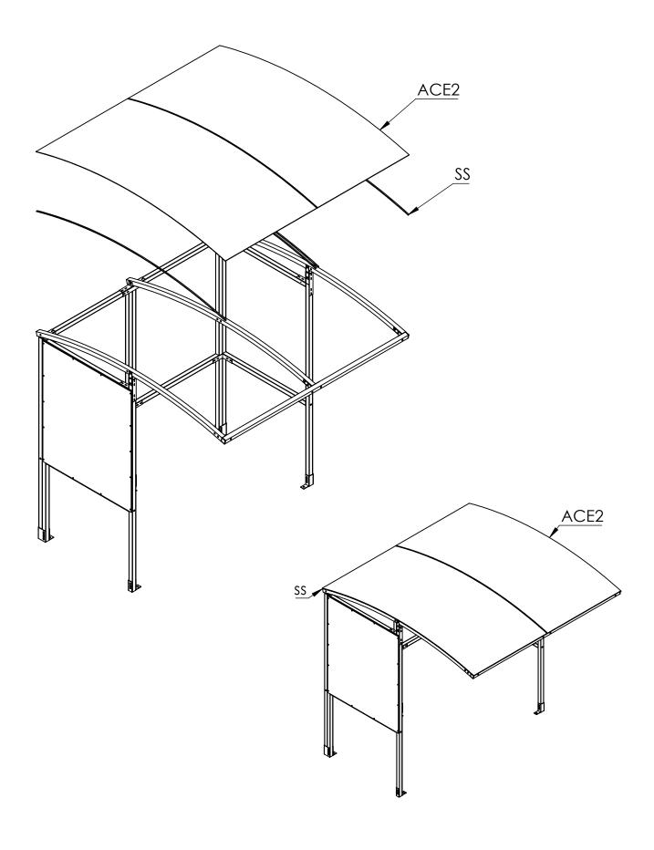
**Step 4** Use **RC2** strips to cover the gap in the centre and the edges and screw them directly into the frame using **25mm TEC** screws. Fit the square end caps **(EC40)** to any open ends of box sections. Screw the **A1 Angle** along the back edge of the roof as shown below.
