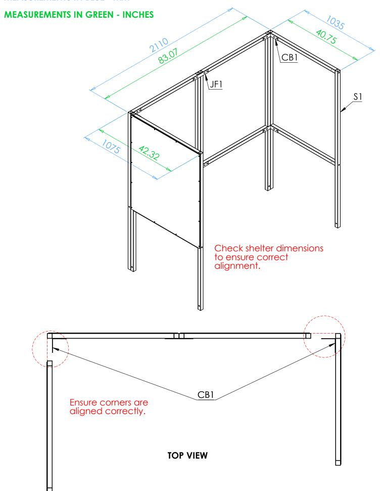
**Step 2** Move the shelter in to its final position, make sure it is square and attach **FT1 and FT3** foot brackets, which screw into the ground using the concrete bolts. Attach **JF2** brackets to **S1** Stubs. Using **CB1** and **JF1** brackets, secure **S1 Stub** to frame. Now fix the **RB1** brackets to the rear of the frame, attach **R4** rafters. Use **L1** brackets to attach **ST8** tie bar.
