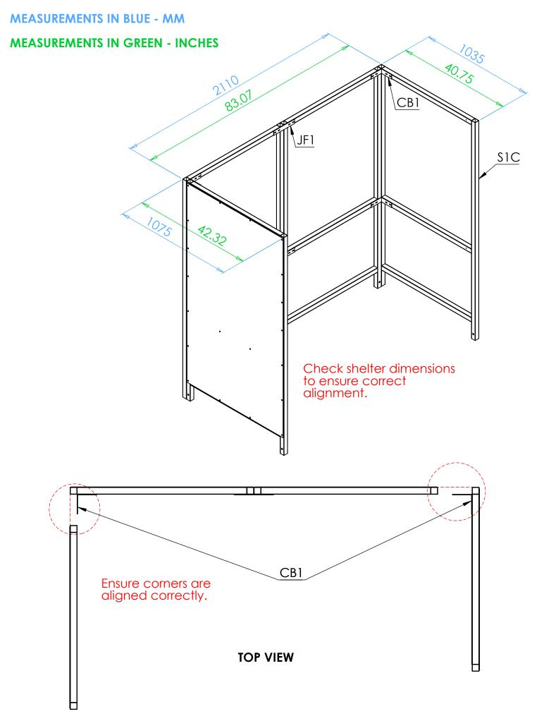
Step 2 Move the shelter in to its final position, make sure it is square and attach FT1 and FT3 foot brackets, which screw into the ground using the concrete bolts. Attach JF2 brackets to S1 Stubs. Using CB1 and JF1 brackets, secure S1 Stubs to frame. Now fix the RB1 brackets to the rear of the frame, attach R4 rafters. Use L1 brackets to attach ST8 tie bar.
