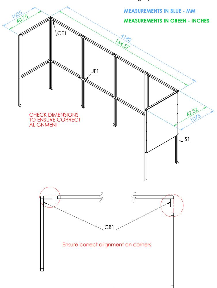
**Step 2** Attach the **S1 stubs** to the front of the frame using **CB1**, **JF1** and **JF3** brackets, then bolt the **R4 Rafter** into place using the **RB1** brackets and the stubs
