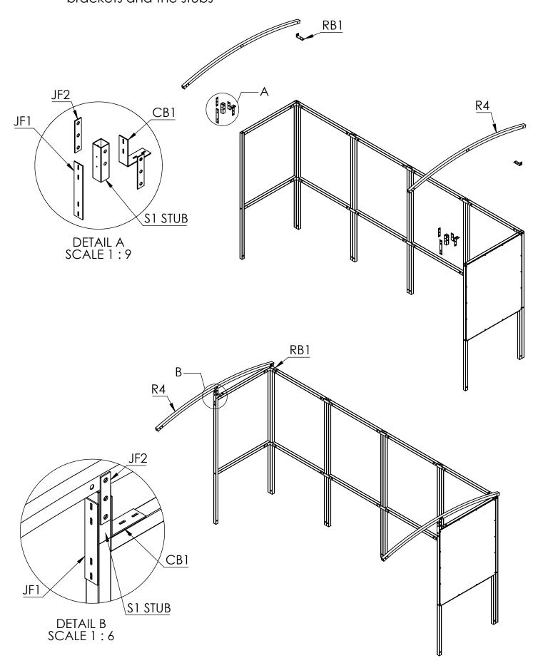
**Step 3** Assemble the T-section by joining the two **ST4** tie bars using a **JF3** bracket then join the **P4** post using two **RB1** brackets and attach a **L1** bracket to each end.
