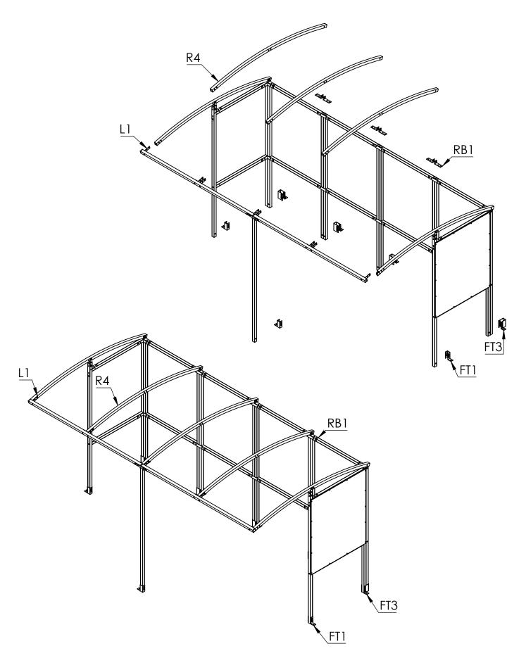
**Step 5** Stick the sealing strips (SS) to the rafters and line up the ACE2 panels with the outside of the shelter then equally space the ACC2 panels in the gap.
