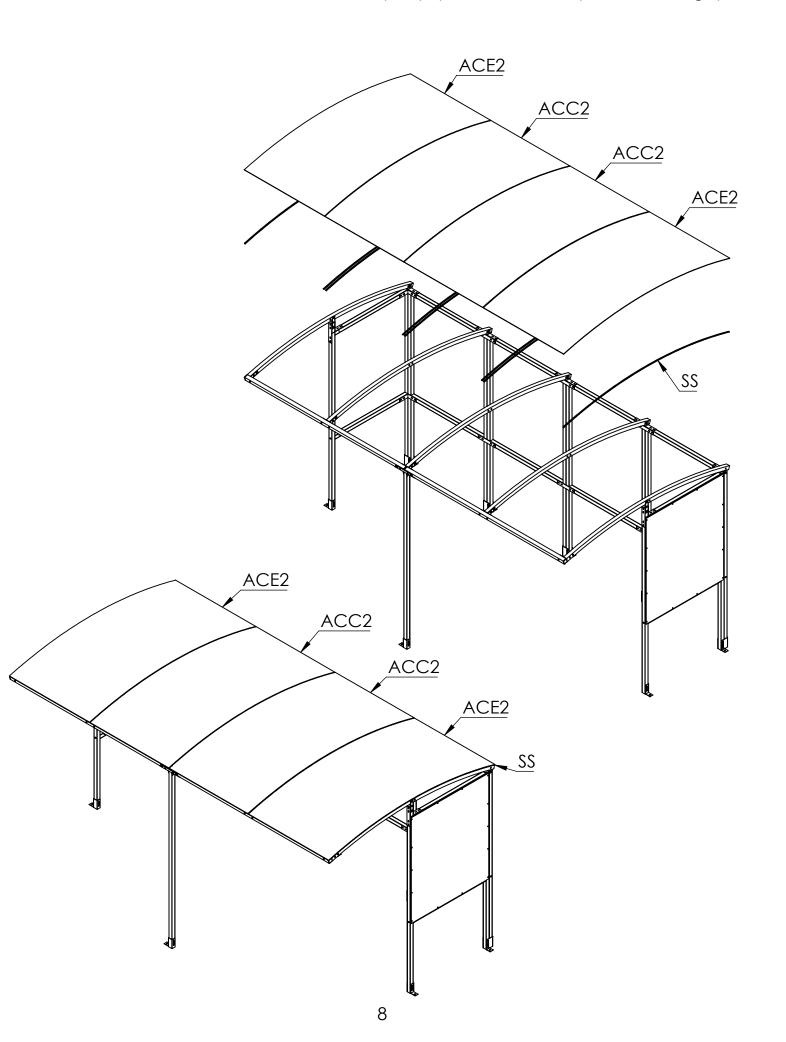
**Step 6** Screw down the **RC2** strips into the rafter with the **25mm tech screws** to secure the roof panels. Push **EC40** end caps into any open ends of box section. Screw **A3 Angle** onto the back edge of the the roof.
