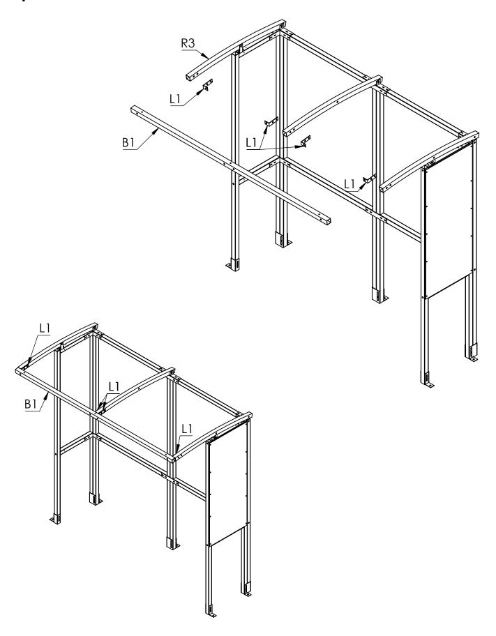
**Step 4** Apply sealing strips to **R3** rafters then put the **PCE1** Panels on top, secure down with **RC1** strips and **38mm Tech screws**. Then attach the **2MD** edge trim.
