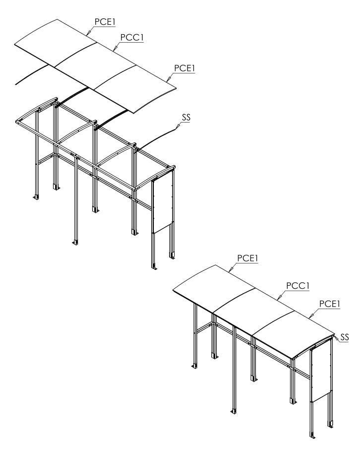
Step 6 Attach the RC1 roof strips, screwing directly into the rafters using 38mm Tech Screws. Push on the 2MD edge trim. Then fit the Black plastic caps on exposed nuts and bolts. Fit the square end caps (EC40) to any open ends of box sections.
