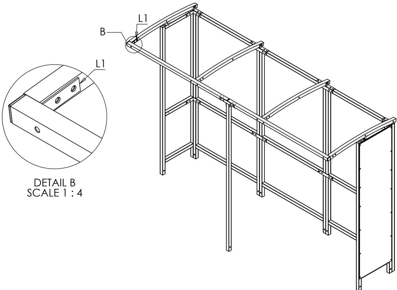
**Step 4** Attach the **FT1** and **FT3** foot brackets, Move the Shelter into its final position and make sure its square. Then use concrete anchor bolts to secure it to the the ground.
