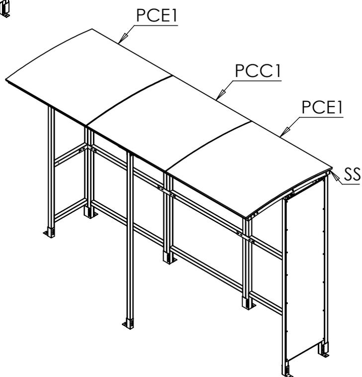
**Step 6** Attach the **RC1** roof strips, screwing directly into the rafters using **38mm Tech Screws**. Push on the **2MD** edge trim. Then fit the Black plastic caps on exposed nuts and bolts. Fit the square end caps (**EC40**) to any open ends of box sections.
