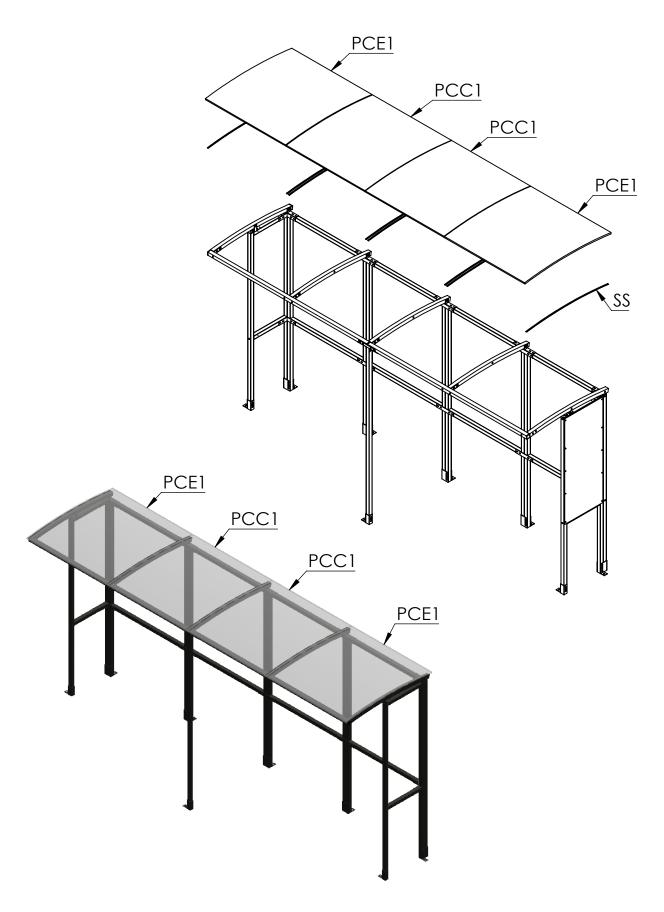
**Step 7** Screw down the **RC1** strips using the **38mm Tech screws** to secure the roof panels in place. Then push the **2MD** edge trim on to the bottom edge of the roof panels. Fit Black plastic caps on exposed nuts and bolts and fit the square plastic end caps to any open ends of box section.
