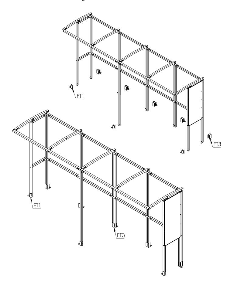
**Step 6** Apply Sealing strips **(SS)** to the rafters and line up the **PCE1** roof panels with the outside of the shelter and equally space the **PCC1** panels between the outer panels.
