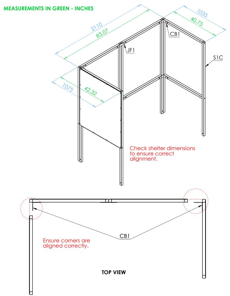
**Step 2** Move the shelter in to its final position, make sure it is square and attach **FT1** and **FT3** foot brackets, which screw into the ground with the concrete bolts. Attach **JF2** brackets to **S1** Stubs. Using **CB1** and **JF1** brackets, secure **S1 Stub** to frame. Now fix the **RB1** brackets to the rear of the frame, attach **R4** rafters. Use **L1** brackets to attach **ST8** tie bar.
