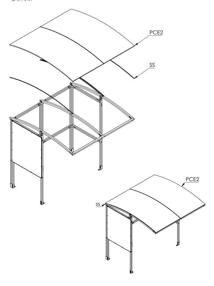
**Step 4** Use **RC2** strips to cover the gap in the centre and the edges and screw them directly into the frame using **38mm TEC** screws. Finish of the shelter by attaching the **2MD** edge trim, then finally, fit the Black plastic caps on exposed nuts and bolts, and fit the square end caps **(EC40)** to any open ends of box sections.
