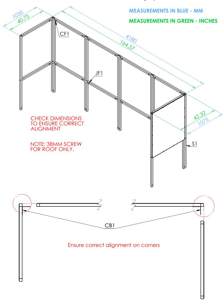
**Step 2** Attach the **S1 stubs** to the front of the frame using **CB1**, **JF1** and **JF3** brackets, then bolt the **R4** rafters into place using the **RB1** brackets and the stubs
