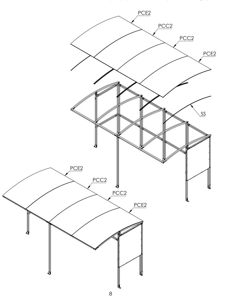
**Step 6** Screw down the **RC2** strips into the rafter with the **38mm tech screws** to secure the roof panels and push the **2MD** end caps on the bottom of the panels.
