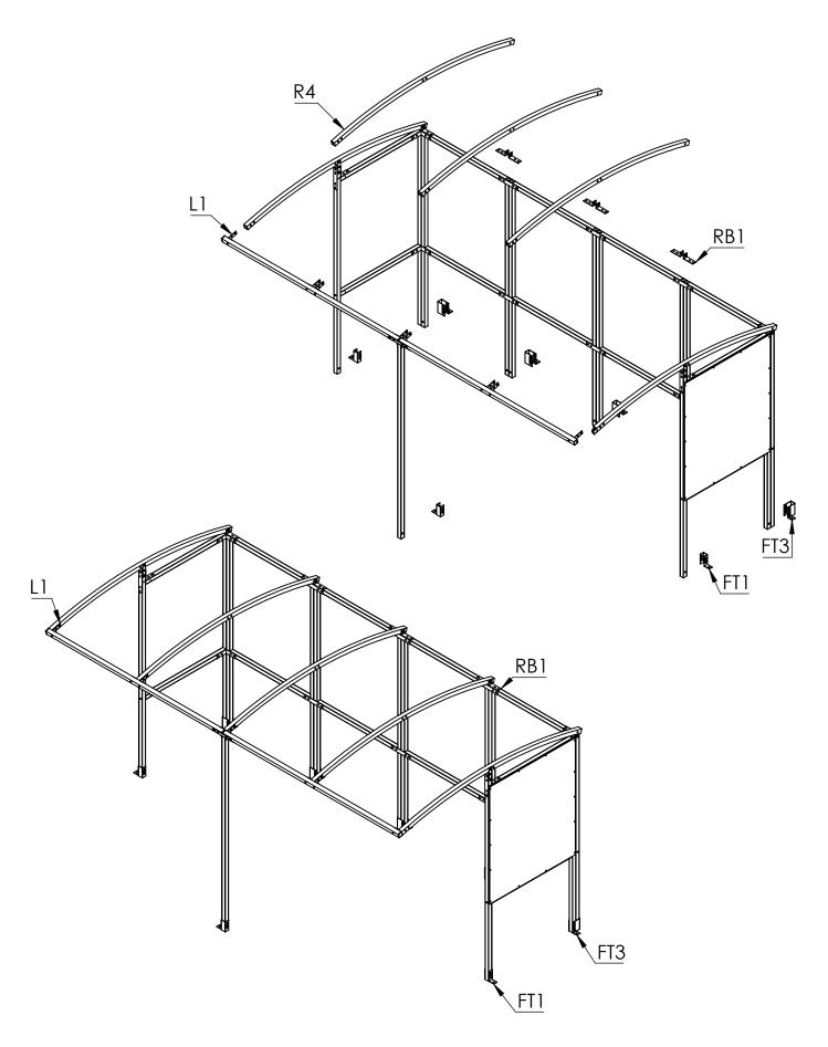
**Step 5** Stick the sealing strips (SS) to the rafters and line up the PCE2 panels with the outside of the shelter then equally space the PCC2 panels in the gap.
